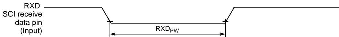
Figure 10-15 RXD Pulse Width
