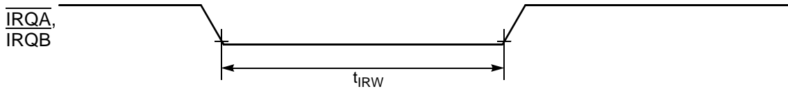
Figure 10-5 External Interrupt Timing (Negative Edge-Sensitive)
