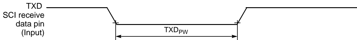
Figure 10-16 TXD Pulse Width
